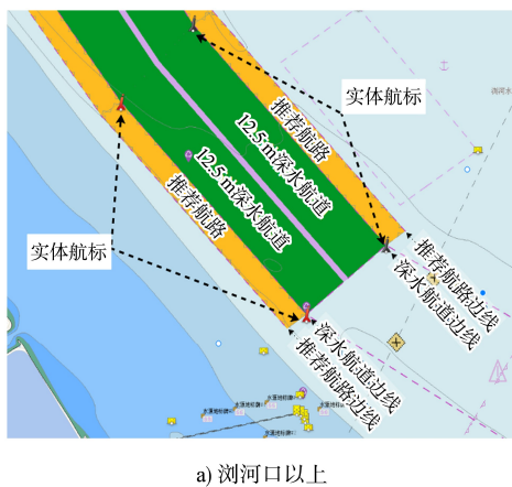
图1 南京以下12.5 m深水航道航标配布横断面 Fig.1 Section of navigation aids on 12.5-meter deep water channel below Nanjing
