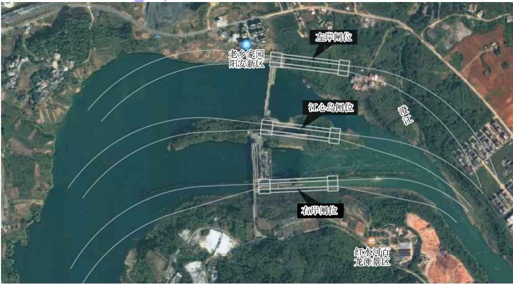
图 2 百龙滩船闸闸位布置 Fig. 2 Position layout of Bailongtan ship lock
