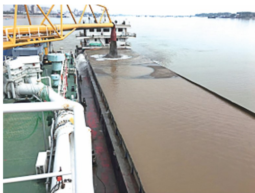
图4 挖砂装驳 Fig.4 Sand-digging and barge-loading
