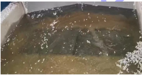
图 8 增加埋深后泄水阀门双边开启时出水口附近流态 Fig. 8 Flow pattern near outlet when water emptying valve is opened on both sides after increasing buried depth
