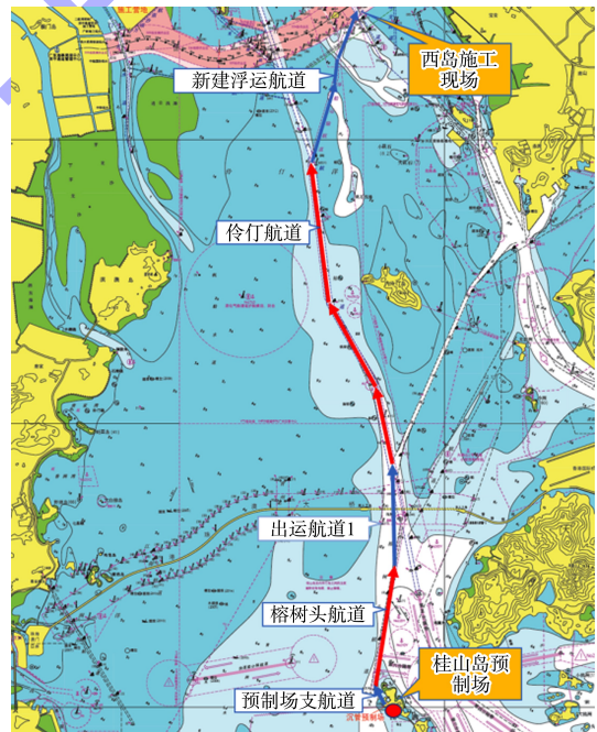
图10 深中通道沉管浮运路线 Fig. 10 Immersed tube floating transportation route of Shenzhen-Zhongshan Link
