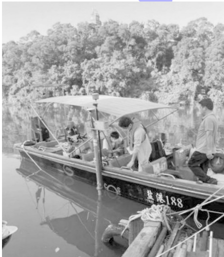
Fig. 2 Installation and testing of multi-beam (first measurement)
