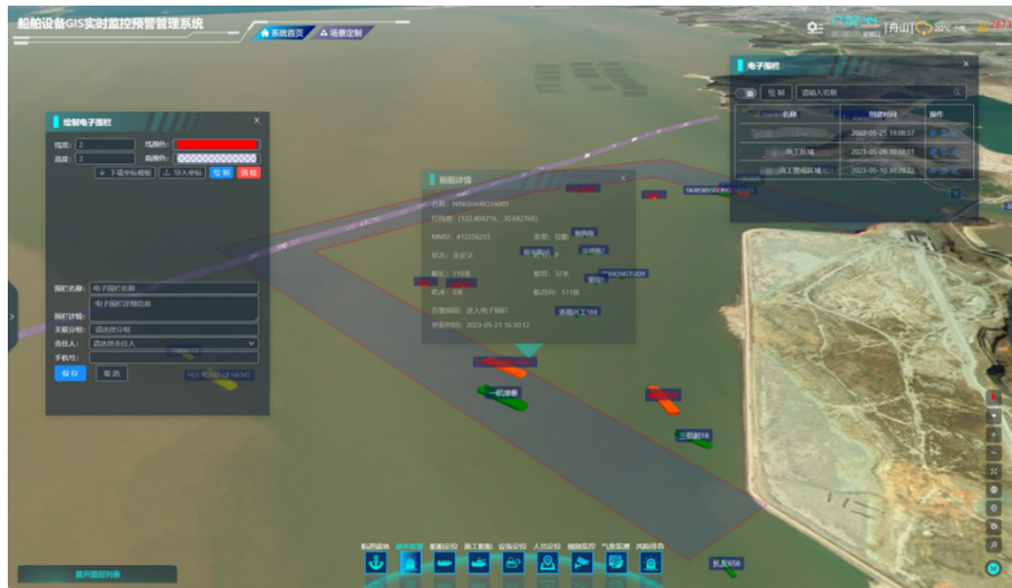
图 7 电子围栏绘制与船舶预警 Fig. 7 Electronic fence drawing and vessel warning
